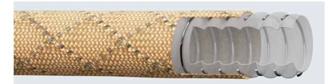
The @marsoflex\* B3 braid is used as a pressure carrier for PTFE hose lines. The braid is made of a polymer which was developed for use as a high-performance fibre and has a high dimensional stability and chemical resistance. Thanks to the interlaced, crossing stainless steel strands (4-8 strands made of 1.4404), an electrical conductivity of <10² is achieved.
